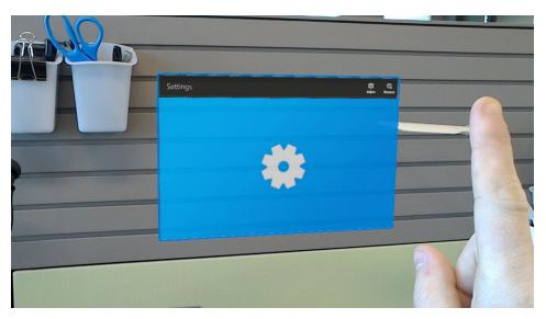
The location and size of the application window can be adjusted by selecting the 'Adjust' button on the top-right corner of the window.
